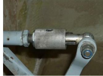
The Wedekind locking sleeve slides outside the l'Hotellier fitting to secure the tab, but doesn't necessarily prevent partial engagement.
