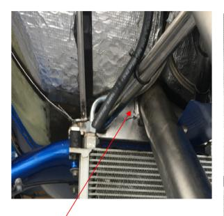
Crack position (could be either side of the mast) between the rear bracket and the mast/keel tube
