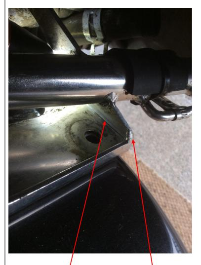
View of crack in the leading edge of the folded bracket area. This is visible from outside front of the bracket. Also check the corner bracket weld
